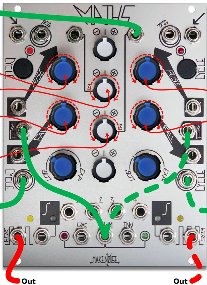
Same as above, only the output is taken from EOC or EOR. CH. 1, RISE parameter will more effectively adjust frequency, and CH. 1 FALL parameter will adjust pulse width. With CH. 4, the opposite is true where RISE adjust more effectively Width and FALL adjust frequency. In both channels all adjustment to RISE and FALL parameters will affect frequency. Use CYCLE IN for Run/ Stop control.
