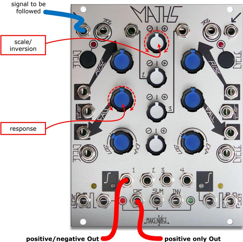
Apply Signal to be followed to Signal IN CH. 1 or 4. Set RISE to NOON. Set and or modulate FALL Time to achieve different responses. Take output from associated channel Signal OUT for positive and negative Peak Detection. Take output from OR buss OUT to achieve more typical Positive Envelope Follower function.
