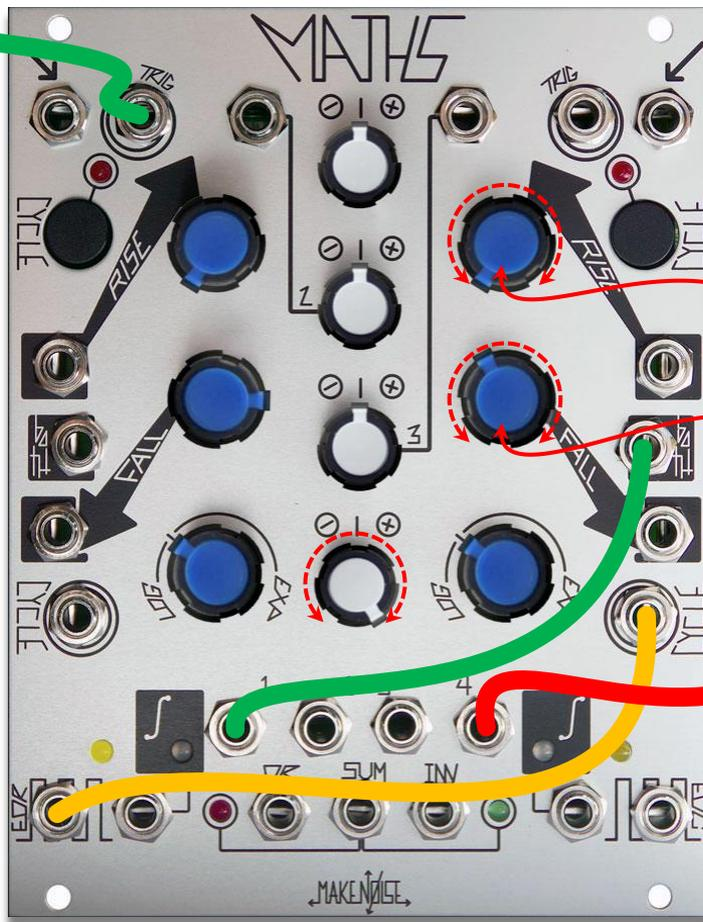
Set CH. 1 RISE full CCW, FALL to 3:00, response to Linear. Set CH. 4 RISE full CCW, FALL to 11:00, response to Linear. Patch CH. 1 EOR to CH. 4 CYCLE In. Patch CH. 4 Output to VCA or LPG control input. Patch a gate or trigger source, such as the touch gate from Pressure Points, to CH. 1 TRIG in. Adjust Channel 4 RISE and FALL for variations.
