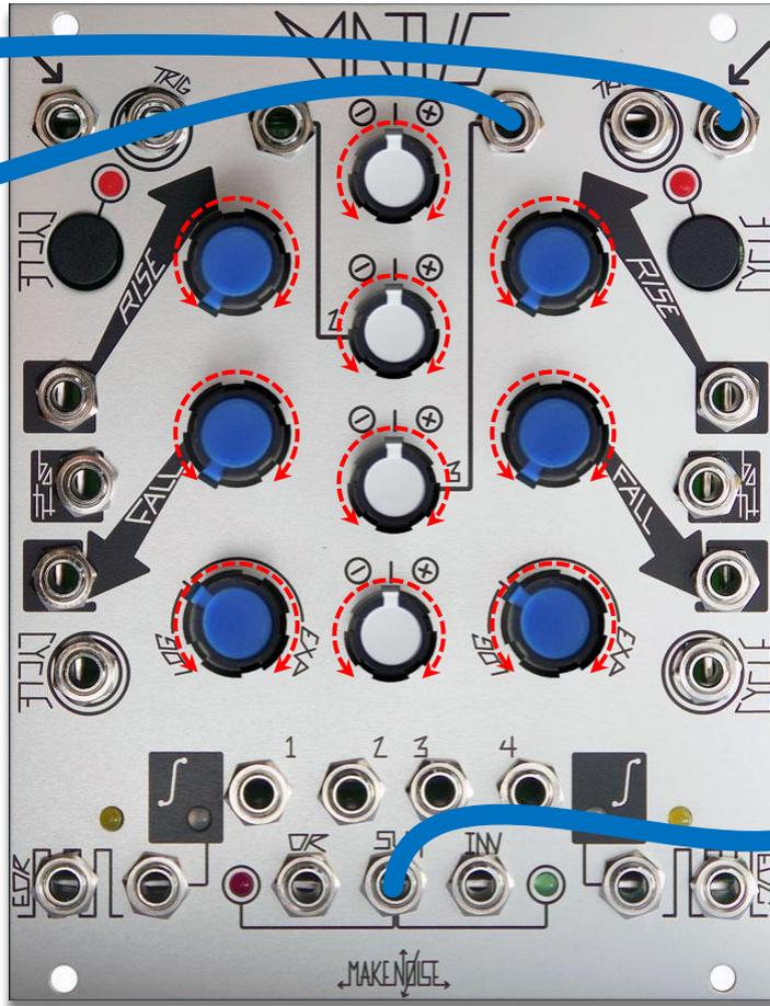
Cycle ch 1 and 4 of Maths by pushing in the cycle button to make them oscillate. Start in Lin mode, and have fall and rise full counter clockwise and adjust from there.
