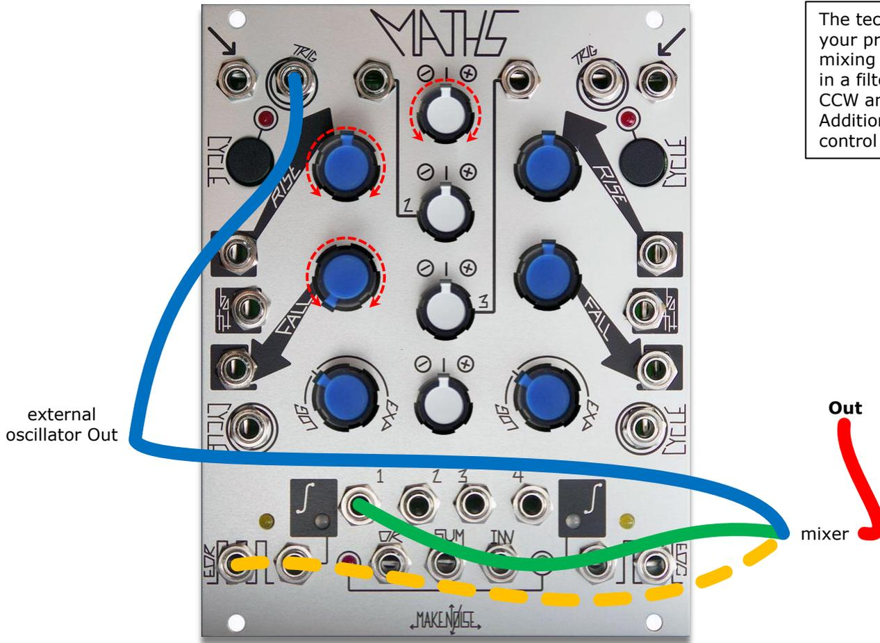
The technique simply involves patching a mult of your principal oscillator to Maths' trigger input and mixing either the envelope or EOR with the main VCO in a filter etc. Set the response to linear, fall to fully CCW and then gradually increase the rise time. Additionally altering the fall time will give you more control over the timing and hence sub-divisions.
