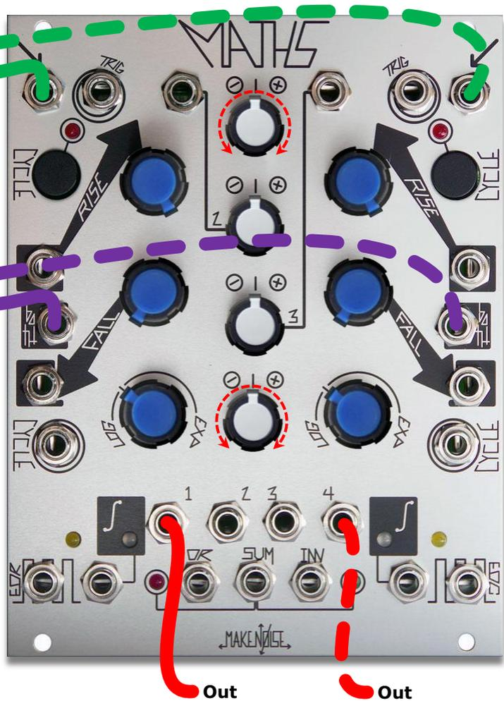
Apply positive going control signal to be multiplied to CH1 or 4 Signal IN. Set RISE to full CW, FALL to Full CCW. Apply positive going, multiplier Control Signal to BOTH Control IN. Take output from corresponding Signal OUT.
