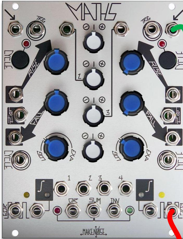
Apply logic gate to CH. 4 Signal IN. Take output from CH. 4 EOC.
