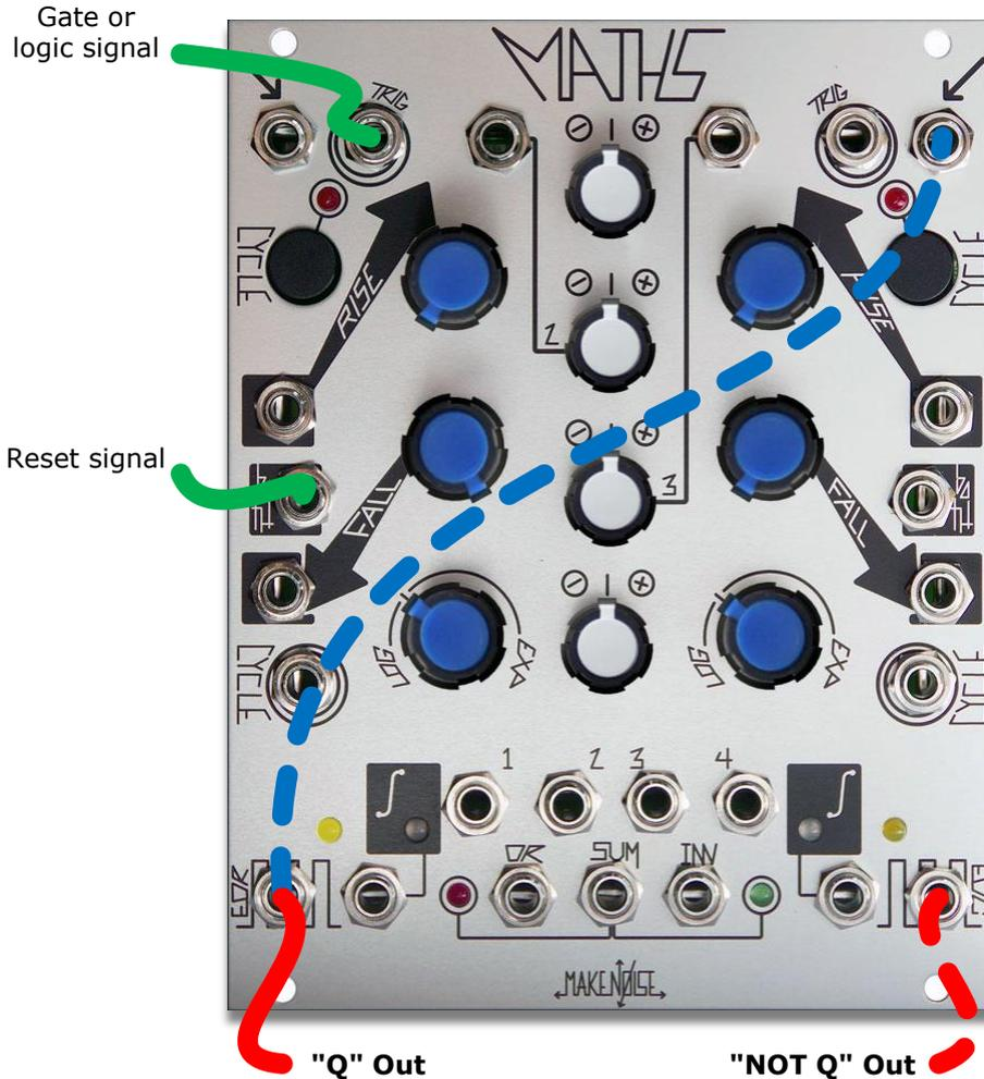
In this patch CH. 1 Trigger IN acts as the "Set" input, and CH. 1 BOTH Contrl IN acts as the "Reset" input. Apply Reset signal to CH. 1 BOTH Control IN. Apply Gate or logic signal to CH. 1 Trigger IN. Set RISE to Full CCW, FALL to Full CW, VariResponse to Linear. Take "Q" output from EOC. Patch EOC to CH. 4 Signal to achieve "NOT Q" at the EOC OUT. This patch has a memory limit of about 3 minutes, after which it forgets the one thing you told it to remember.
