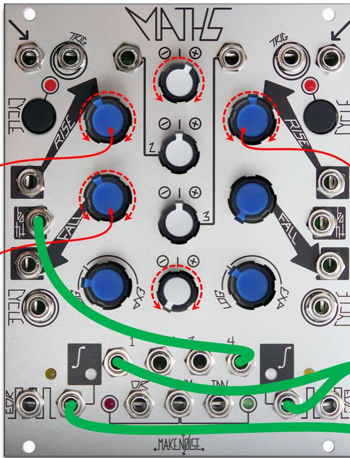
Maths Channel 4 set up as fast square-ish LFO (Lin curve, mid Rise, zero Fall, full negative negative output)
