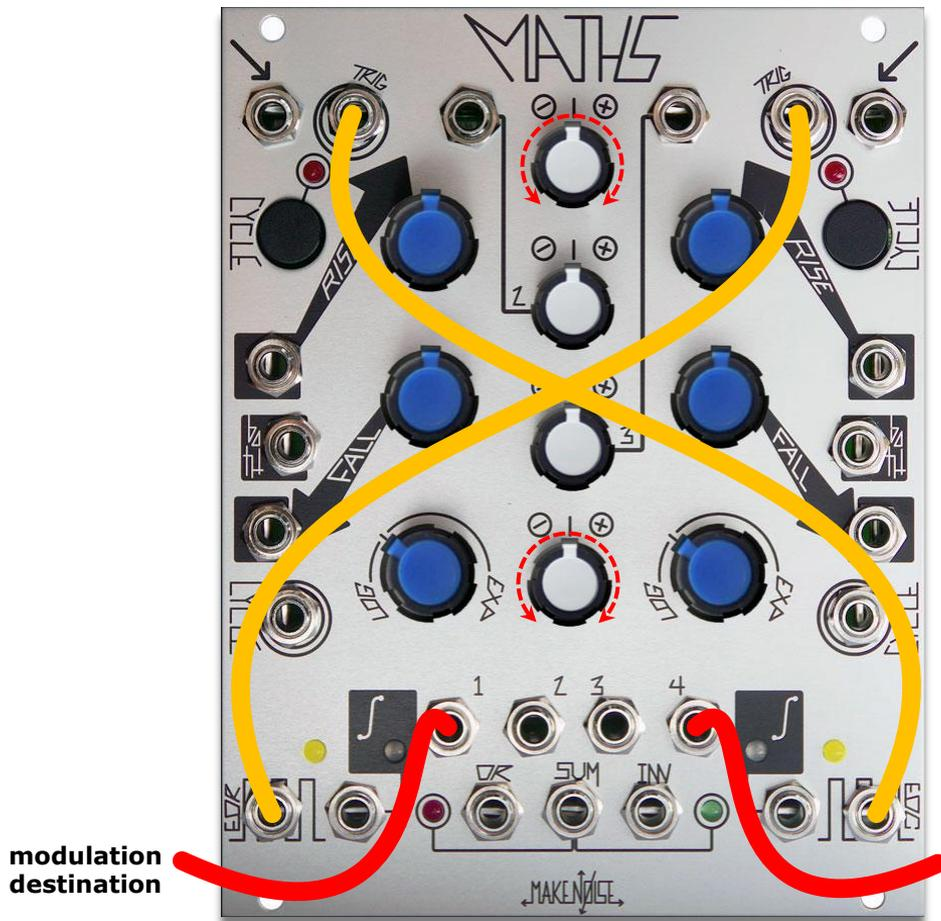
In this patch, CH. 1,4 work in tandem to provide functions shifted by ninety degrees. With both Cycle Switches UNENGAGED, Patch End of RISE (CH. 1) to Trigger IN CH. 4. Patch End of Cycle (CH. 4) to Trigger IN CH. 1. If both CH.1 and 4 do not begin cycling, engage CH. 1 CYCLE Briefly. With both channels cycling, apply their respective Signal outputs to two different modulation destinations, for example two channels of the Optomix.
