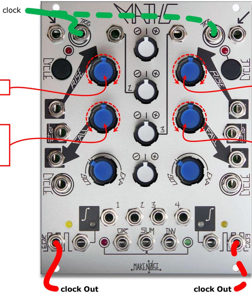
Clock signal applied to Trigger IN CH. 1 or 4 is processed by a divisor as set by RISE parameter. Increasing RISE sets divisor higher, resulting in larger divisions. Fall time will adjust the width of the resulting clock. If the Width is adjust to be greater the the total time of the division the output will remain "high."
