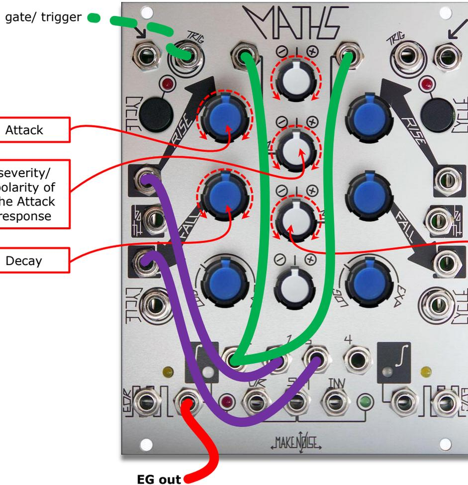
By changing the level and polarity of the Variable OUT of CH. 1, 4 with the Attenuvator, and feeding that signal back into CH.1, 4 at RISE or FALL Control IN, independent control of the corresponding slope is achieved. Take output from Unity Signal OUT. Best to have the Response panel control set to NOON.
