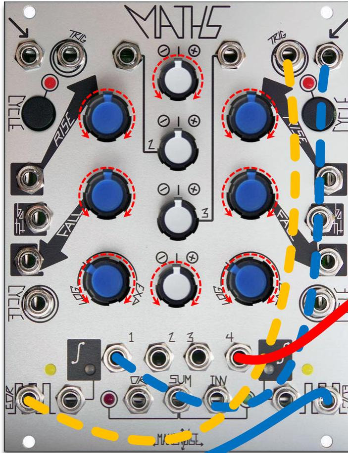
Set channel 4 to self cycle at audio frequency and route the output to your mixer.
