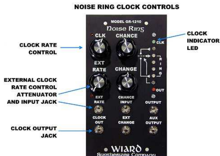
Clock controls on the Model 1210.
